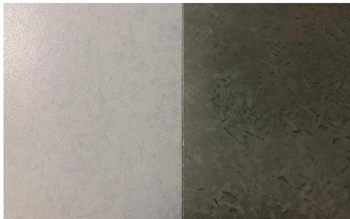
圖 3. Figure 3. 建議塗層的厚度(左) vs GI 表面(右) Coating with recommended thickness (Left) vs naked
