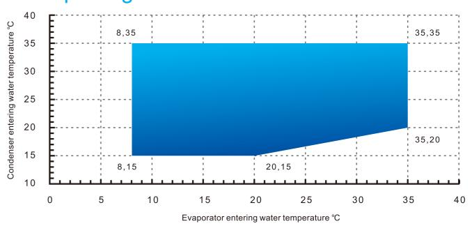
Notes: After the chiller is started, condenser inlet water temperature must be higher than evaporator inlet water temperature within 5 minutes. If not, please add a bypass valve in condenser inlet water pipe.
