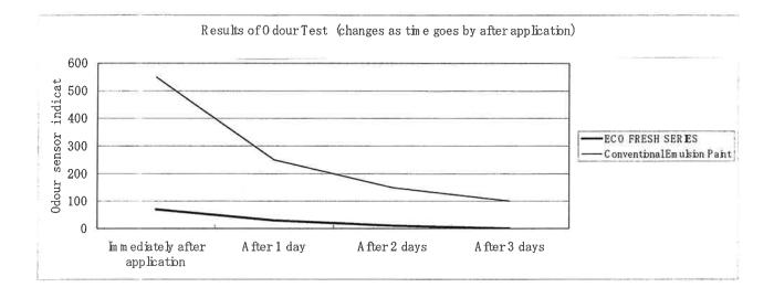
Odour was measured with a sensor at each testing time after application on an internal wall.
