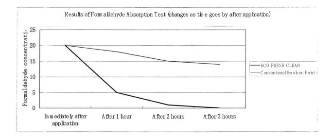
Formaldehyde concentration was measured with a gas detecting tube at each testing time after a test piece was put in a 3-litter container of 20ppm concentration of formaldehyde.
